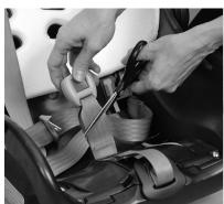
Remove and discard Remove and discard harness webbing and mixed plastic/metal components.
